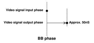
2) Video signal input phase (frame synchronizer is ON)
